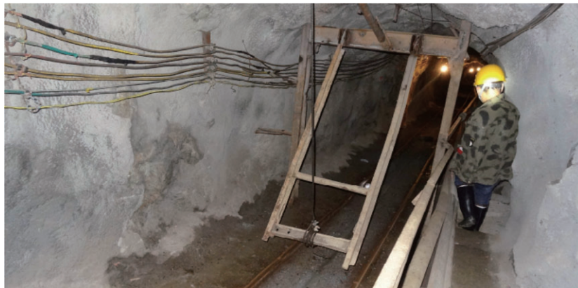
Figure 5-5: Blind Incline Shaft (Real of the mine, photo took in June 2023 by APA)
